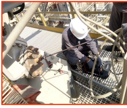
Stack Emission Testing
