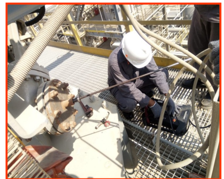
Stack Emission Testing
