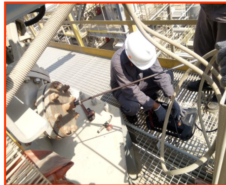
Stack Emission Testing
