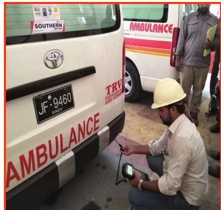
Vehicle Emission Monitoring
