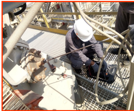
Stack Emission Testing
