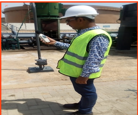
Noise Monitoring in Plant Area
