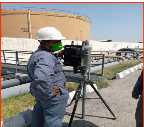
Fugitive Emission Testing
