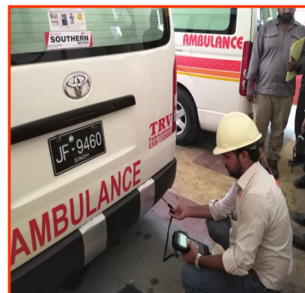
Vehicle Emission Monitoring
